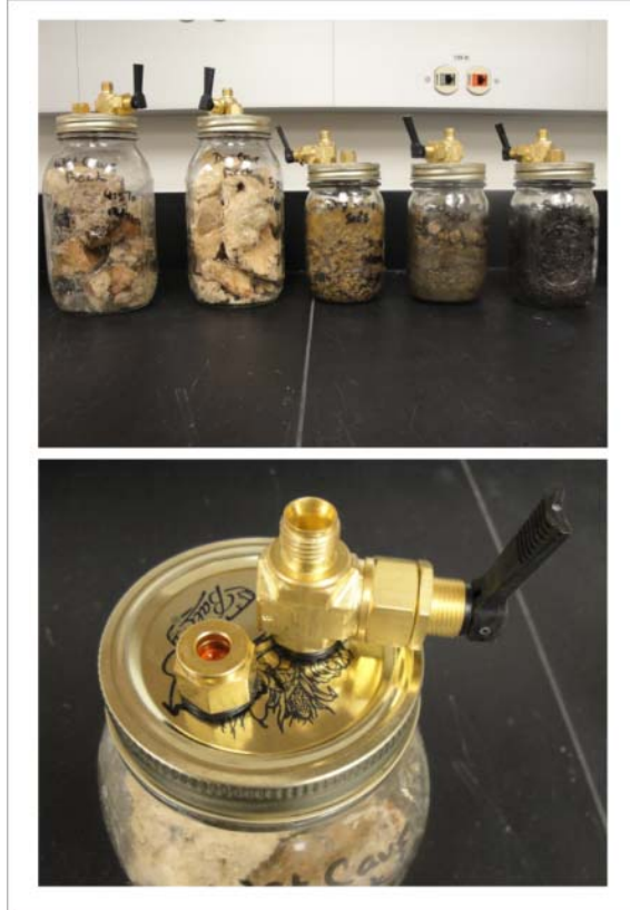
Figure 3.4. CO 2 respiration chambers. Bottom: close-up of Swagelok® valve and septa.
